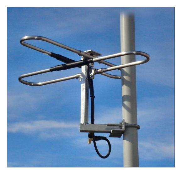
Double dipole omni directional turnstile antenna composed of aluminum, complete with a hot dipped galvanized steel mount. The antenna is frequency tuned on channel for minimum VSWR and maximum efficiency in the 174 – 216 MHz spectrum.
